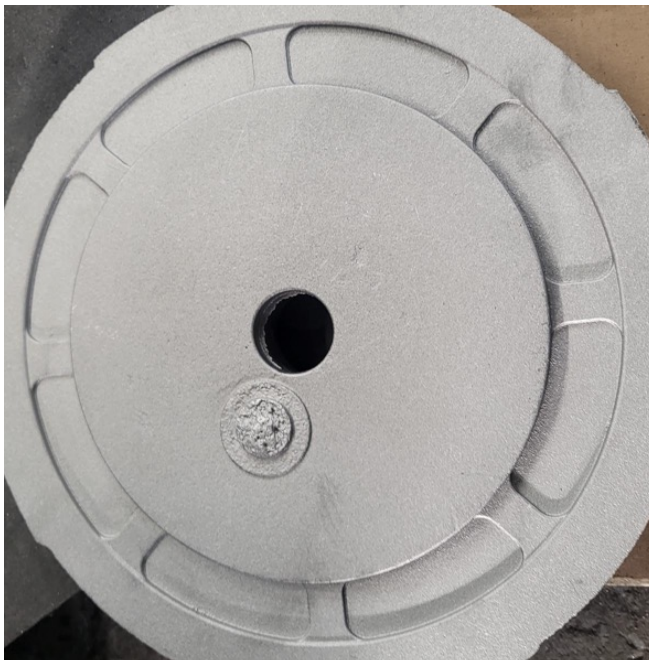
Figure 13. shows the improved final casting finish after the smaller insulated feeders were applied.
